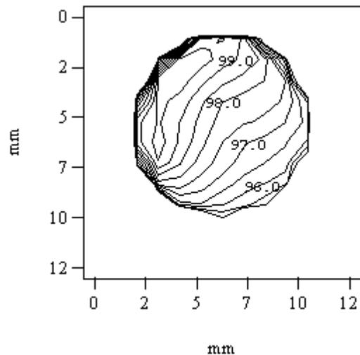
**Fig. 2:** Uniformity tested at 240nm of UV enhanced photodiode used by NIST as a transfer standard for 200nm to 400[1]
