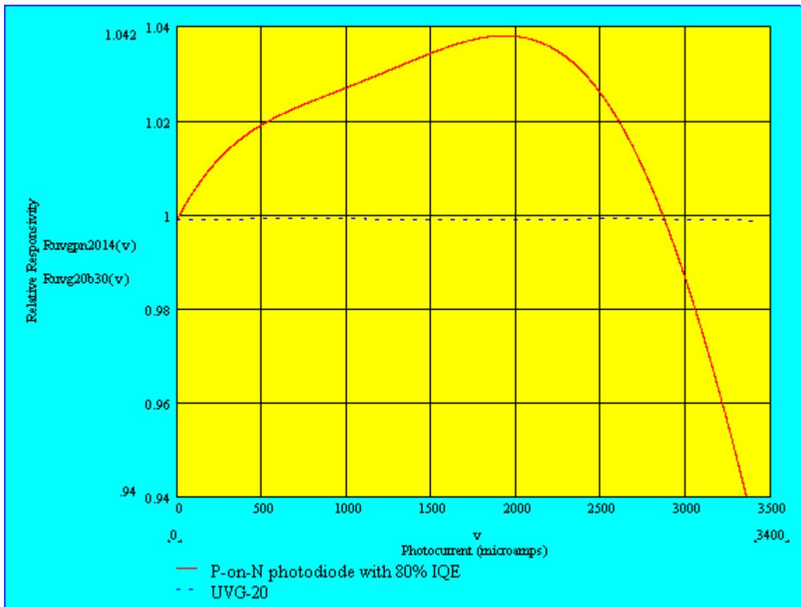
**Fig. 2:** Linearity of P-on-N photodiode with 80% internal quantum efficiency and UVG-20 photodiode with 100% internal quantum efficiency.
