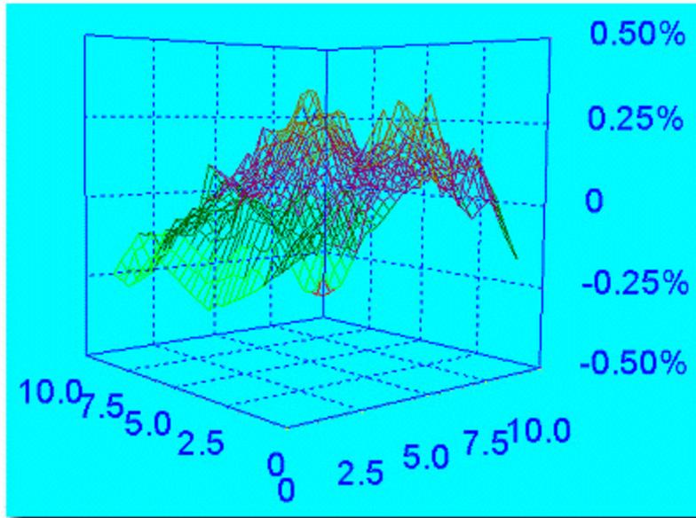
**Fig. 1:** Uniformity of UVG-100 photodiode at 254 nm.
