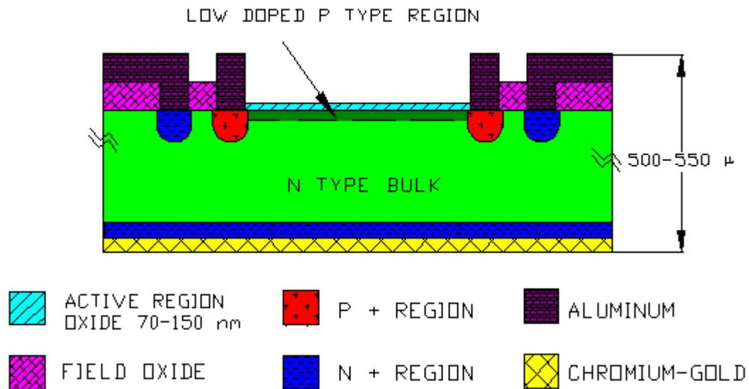
**Fig. 4:** Structure of the UVG-PN20 photodiode
