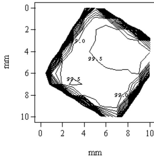
**Fig. 1:** Uniformity of IRD photodiode at 240 nm [1].
